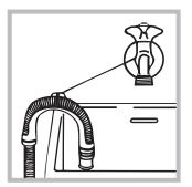
If it is place over the edge of a basin or sink be sure the free end of the hose should not be underwater.
